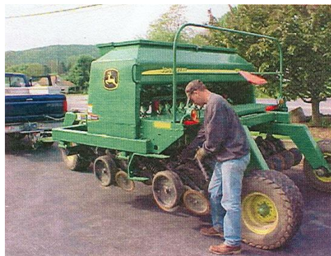
Technician Jared Shippey greasing drill.
